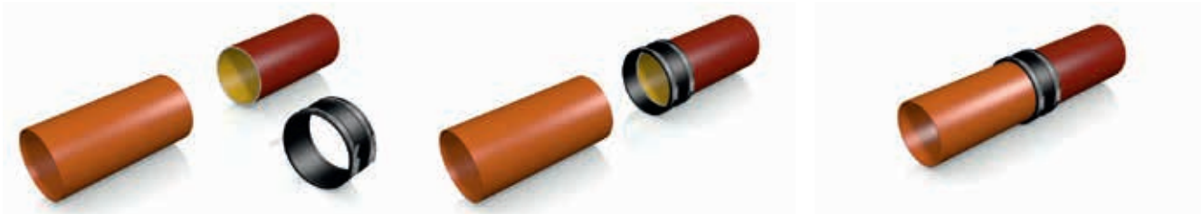
Position plain ended pipes.
