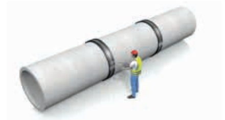
Center coupling over joint. Tighten clamps and shear band reciprocally.
