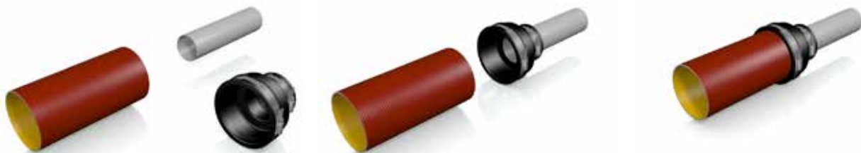
Position plain ended pipes.
