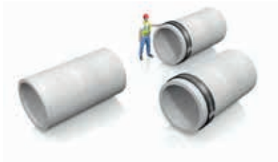
Position plain ended pipes.
