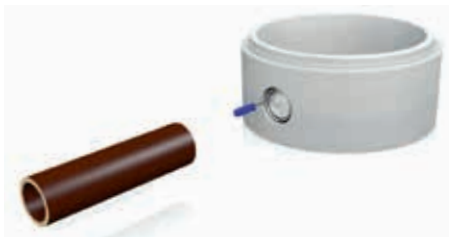
Remove polystyrene from socket.
